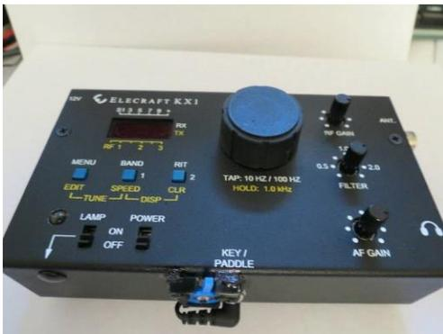
Pictured is the installed paddle wired to a stereo plug.
