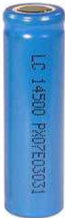
The battery shown is sold by Batteryspace.com. Each bank would have three 3.7v batteries in series. As each battery can produce 750MAH, thus one bank produces 11.1v @ 750MAH. I then put each battery bank in parallel. I now have an internal battery for my KX1 that will produce approximately 12v @ 1.5AH. Yes the three 3.7v batteries in series of each bank have a working voltage of 11.8 VDC. This will produce around 4w of RF power from my KX1.
