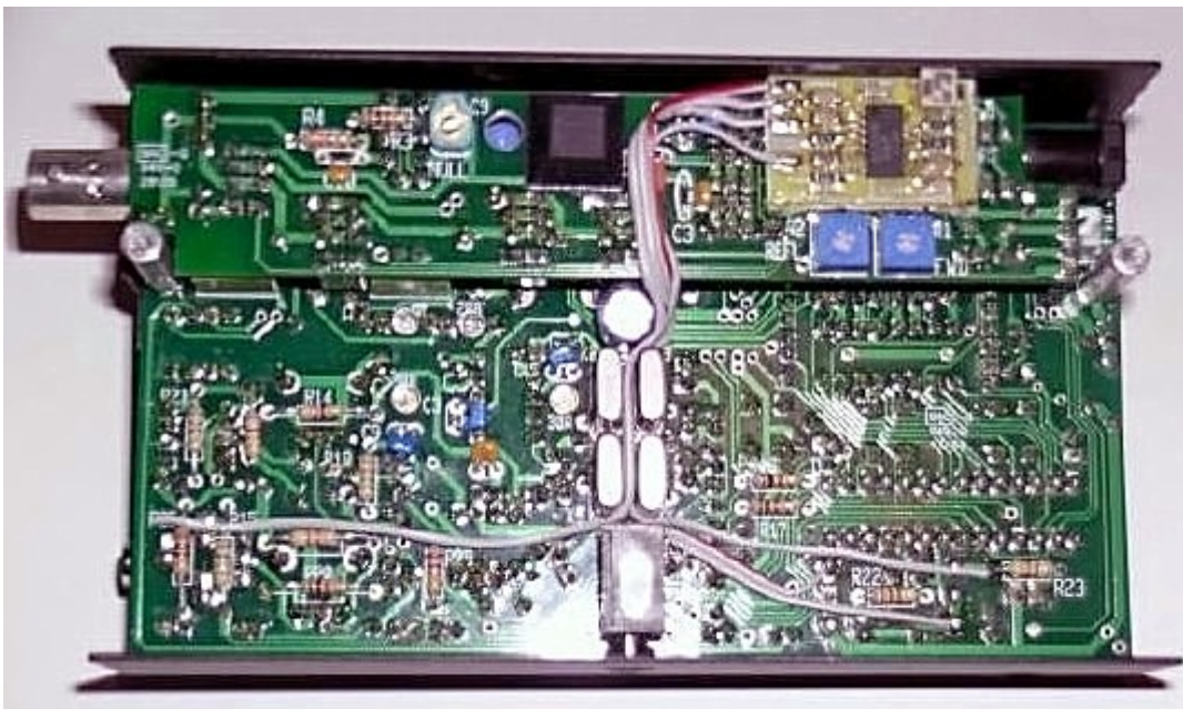
K6XX SMD CW Indicator installed on top of the ATU in my Elecraft KX1.
