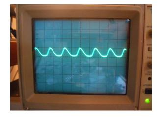
I now just touch up C40 so it's dead on at 10.116mhz. At this point I have a working Cub with a FCC-2 DDS VFO wired to it with the analog VFO taken out
