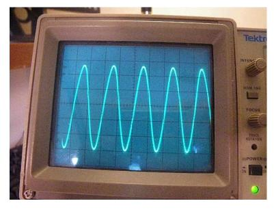
I check the Low –Z Output of the FFC-2, but it's just too much signal there. Even with the gain pot turned completely down I have around 1V p/p output. But, it's a nice clean-looking signal. Now I have to find a lower output or build an attenuator. I also set the FCC-2 to RX-IF and Mode and RX IF =6mhz. This will give me a 4.100mhz to 4.150mhz signal that I need since the cub has a 6mhz IF in it.
