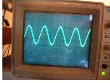
The DDS VFO 4mhz signal from the FCC-2 goes to Q4 and then to transmit gain pot R19. From there into TX Mixer U5. Here the 4mhz signal mixes with the 6mhz signal to produce a 10mhz signal. I did not change anything in this circuit. I did have to adjust R19 in the Cub down a bit, but not much. I also retuned L6 and L7, but they really didn't need it.
