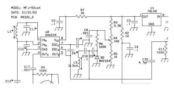
I now proceed to remove VFO components C6, C7, C9, C10 and D2. This isolates VFO U2 pin 6 and pin 7. It also insolates the pot R6 which I might use as a keyer speed adjustment pot. I leave L3 on the board as it's just to hard to remove this coil. I did check the VFO output level before removing the parts and it's about 150mv p/p at U2 Pin 6.
