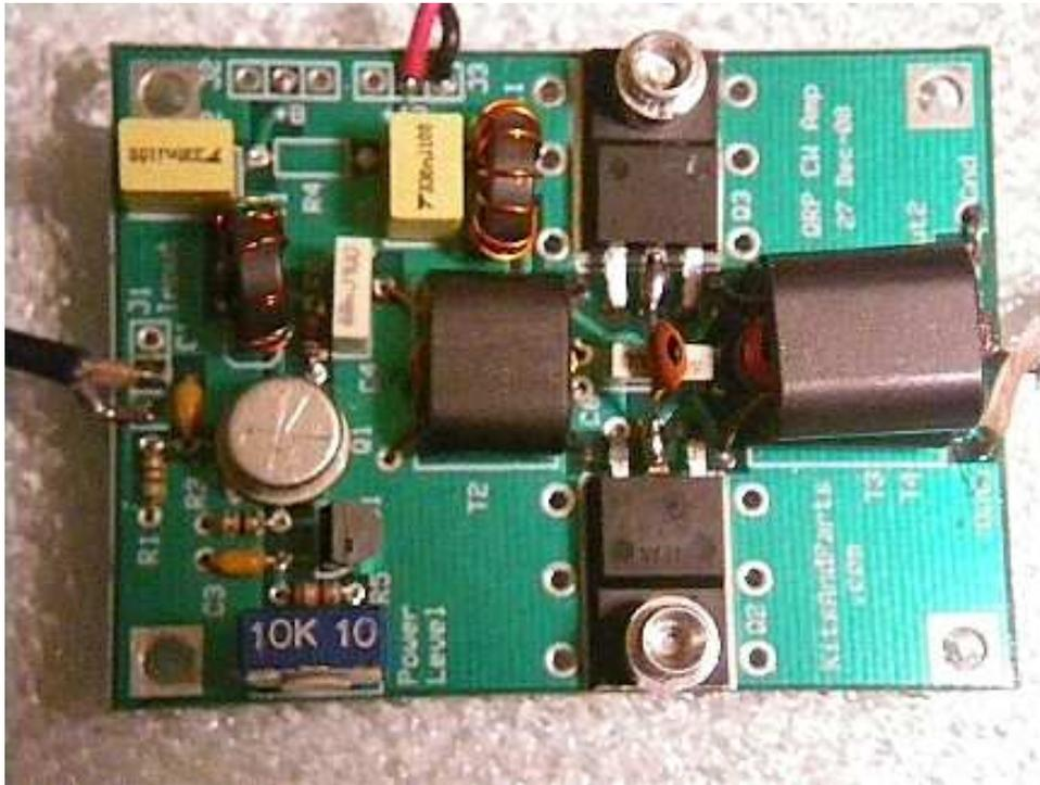
Shown above is the QRP 5W Amp Kit I purchased from [Parts and Kits.com](http://Parts and Kits.com). The kit sells for \$18.00 and has a low part count. I found the kit easy to build except for one thing. The website picture for winding T2 was correct, but the text was wrong. Except for that, the kit was easy to build.
